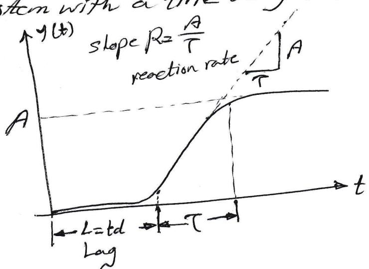
Ziegler and Nichols gave two methods for tuning PID controller for such a model. In the first method the choice of controller parameters is designed to result in a closed-loop step response transient with a decay ratio of approximately 0.25. This means that the transient decays to a quarter of its value after one period of oscillation.
