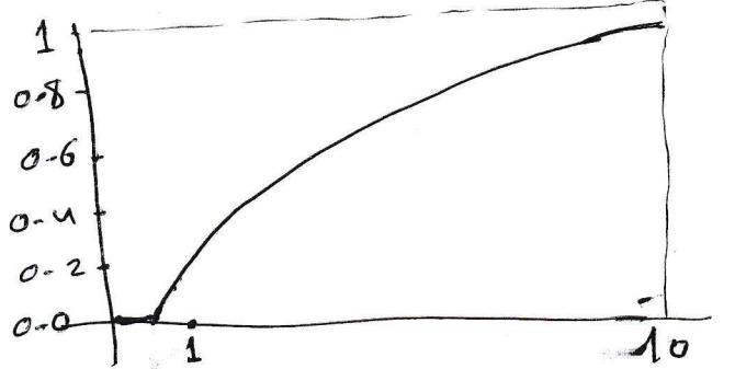
Find the proportional P, PI, and PID controller parameters by using the Zeigler - Nichols transient-response method.
