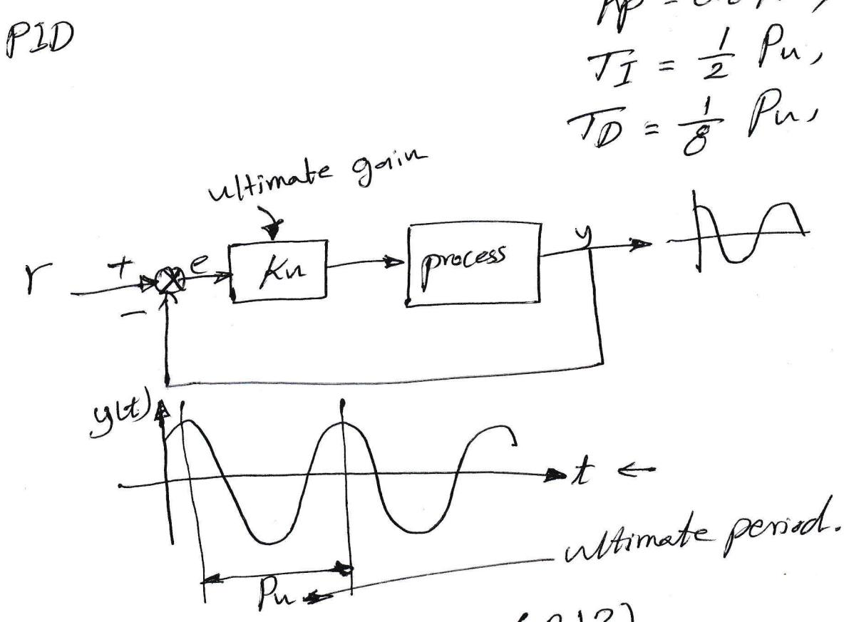
E<sub>x</sub> if you have a system with ultimate gain  $K_u = 15.3$  and the period is measured as shown in figure below. Determine the proportional and PI regulators according to the Ziegler-Nichols rules based on the ultimate sensitivity method.
